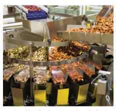
WeighPack's 24 head PrimoCombi multi-head weigher with three product mixing weighs product before it is bagged.
