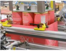
Eagle Packaging Machinery's Pick & Place Automation precisely loads each Roca container into the case while simultaneously orienting all logos to ensure that shipments are retail-ready.
