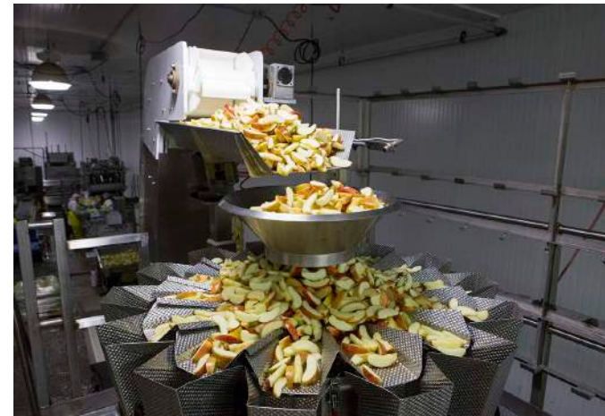
The robust 14-head PrimoCombi weigher from WeighPack Systems accurately portions apple slices by weight into buckets to distribute into a Swifty Bagger 3600 (below).
