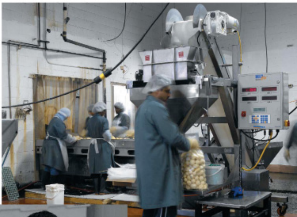
The Tiger Scales IW-25 machine from WeighPack Systems plays a pivotal, central part in the packaging of peeled potatoes at Vegfresh, handling an average of 100 bags per hour.
