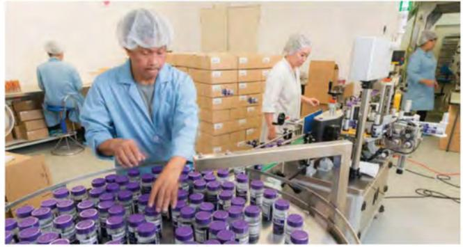
A WeighPack Systems complete solution automatically conveys, weighs and fills containers with its unique SpinDexer rotary indexing system designed specifically for vitamin gummies.
