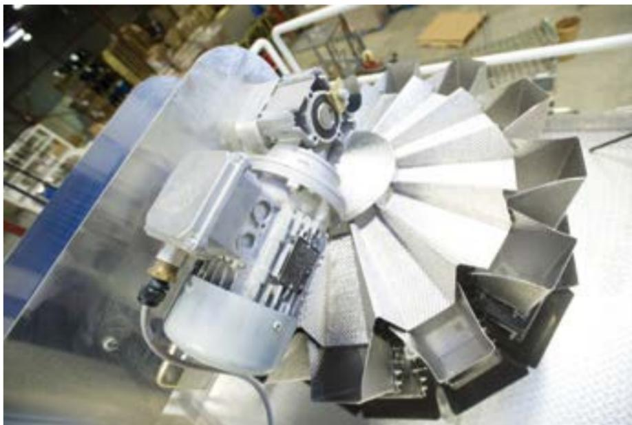
High-precision 14-head Multiweigh scales installed by RJP Packaging are used to dispense precise quantities of dishwashing detergent pods down to the packaging lines.
