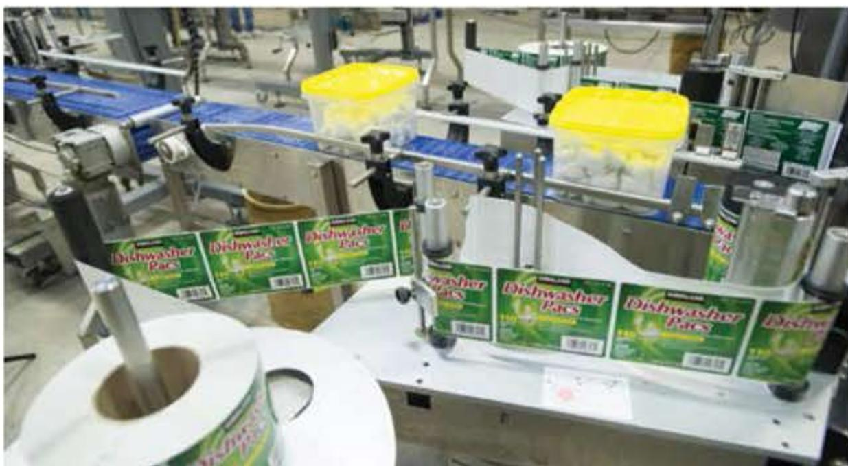
A high-speed model SPM-10 side wipe-on label applying system manufactured by Speedway Packaging Machinery swiftly applies pressure-sensitive product labels onto the side panels of plastic tubs with exacting placement precision.
