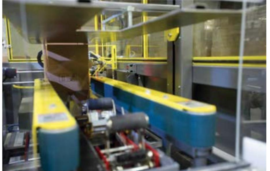
A close-up view of the Eagle Packaging Machinery's case-erector feeding the JemPak packaging lines with corrugated shipping boxes made by Atlantic Packaging Products.
