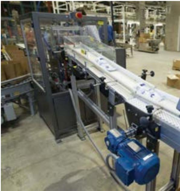
A heavy-duty SEW-Eurodrive motor (*foreground*) powers the Speedway conveyors transferring stand-up pouches inside the Eagle Packaging collating machine.
