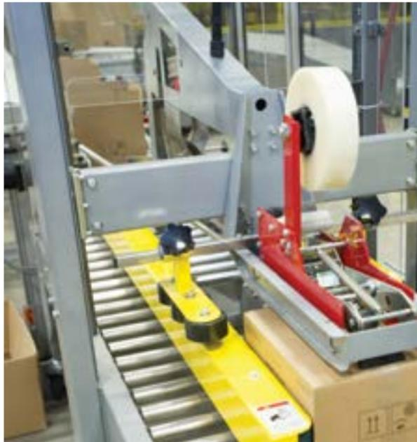
An automatic case-sealing machine from Eagle Packaging Machinery applies strips of high-strength sealing tape onto the top of each passing corrugated box.
