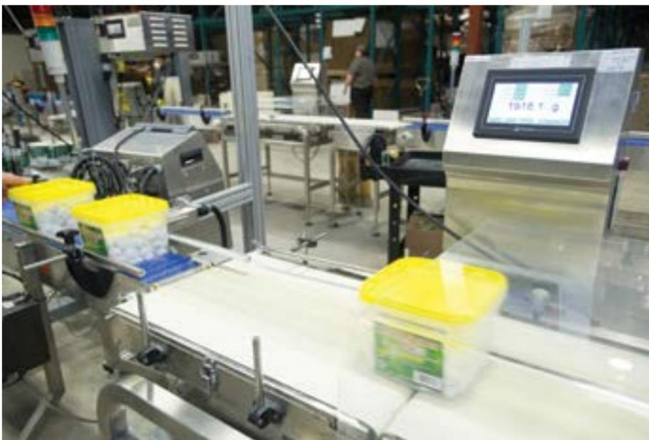
A Multiweigh checkweigher installed by RJP Packaging verifies the weight of plastic tubs used to package larger quantities of detergent pods preferred by Big Box retail customers.
