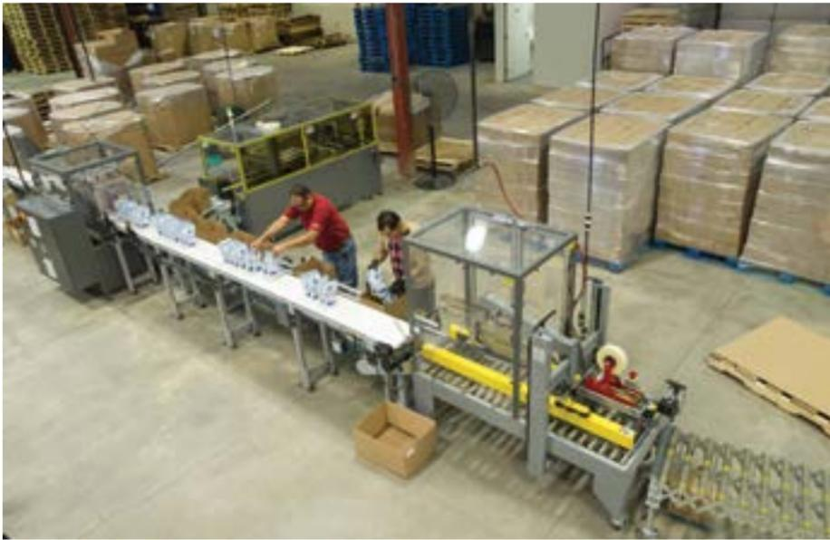
A bird's-eye view of one of the plant's two highly-automated packaging lines utilizing high-speed collating, box-erecting and case-sealing equipment from Eagle Packaging.
