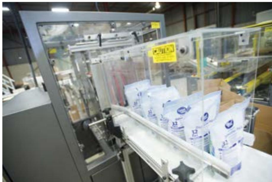
Precise quantities of filled stand-up pouches of dishwasher detergent pods making their way out of the fully-automatic collator manufactured by Eagle Packaging Machinery.
