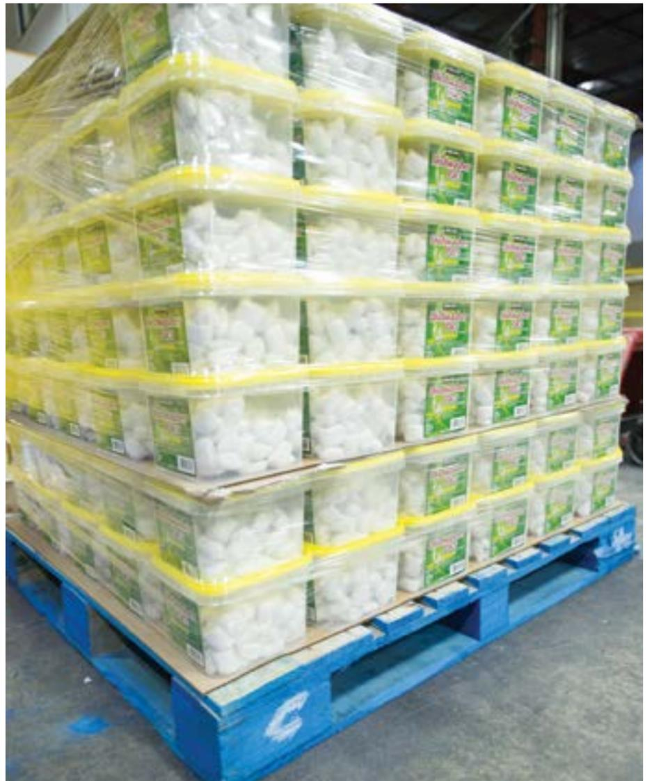
The stackable plastic tubs used to package larger quantities of dishwasher detergent pods for Big Box retail customers help to ensure optimal cube utilization during transit.
