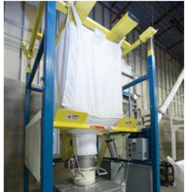
A heavy-duty woven super sack filled with bulk powder detergent blend is prepped up for discharge and processing into monodose, single-use dishwashing detergent tablets.
