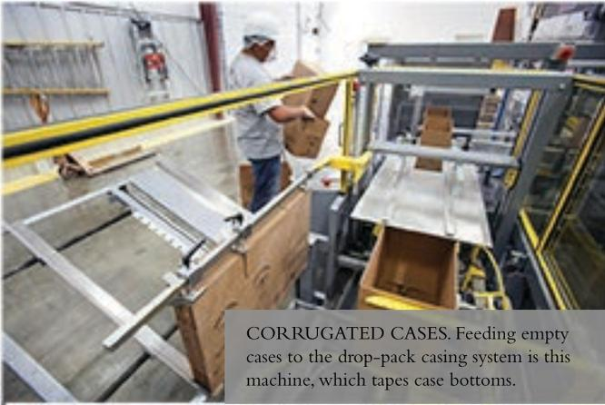
**CORRUGATED CASES.** Feeding empty cases to the drop-pack casing system is this machine, which tapes case bottoms.
