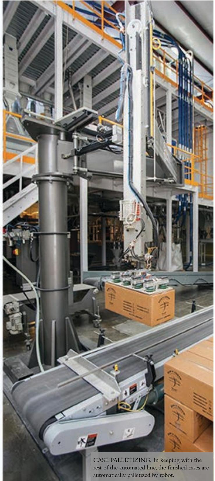
**CASE PALLETIZING.** In keeping with the rest of the automated line, the finished cases are automatically palletized by robot.
