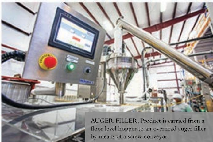
**AUGER FILLER.** Product is carried from a floor level hopper to an overhead auger filler by means of a screw conveyor.
