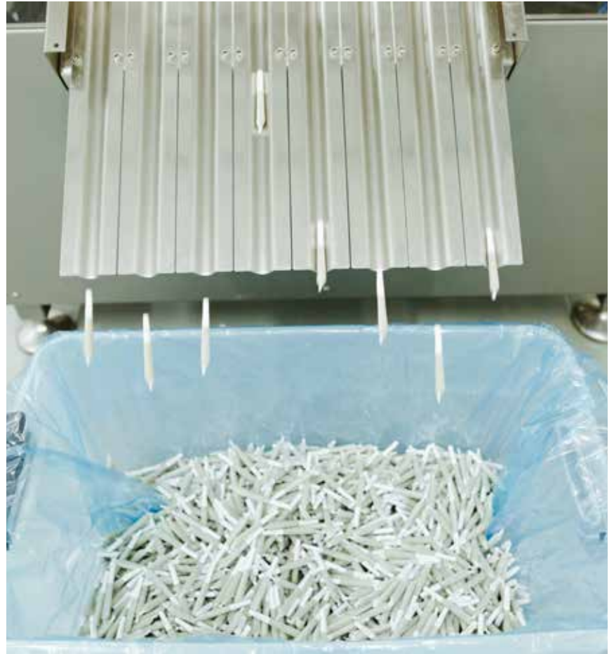
Featuring a unique inline design, the eight-channel JuanaRoll installed at the Crossfield plant can produce up to 50 pre-rolled cones of uniform size and weight in one single pass whereby the machine automatically fills, compacts, tamps, twists, trims and ejects the finished pre-roll into the plastic basket below at the machine's back end.
