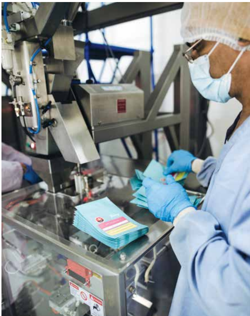
Clockwise from left A plant employee preparing to load pre-made pouches onto the Swifty Bagger Mini machine; machine operator loading pre-made paper cones onto the front end of the eight-channel JuanaRoll machine; rows of bulk Futurolla pre-made paper cones taken out of the box for loading the JuanaRoll machine.
