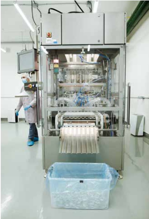
Featuring a unique inline design, the eight-channel JuanaRoll installed at the Crossfield plant can produce up to 50 pre-rolled cones of uniform size and weight in one single pass whereby the machine automatically fills, compacts, tamps, twists, trims and ejects the finished pre-roll into the plastic basket below at the machine's back end.
